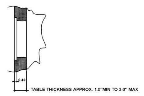
NOTE: Specifications subject to change without notice. Always confirm measurements before cutting to ensure that specifications have not changed. Always make sure to orient cutout in direction necessary for proper operation of the installed unit. Tolerance: ± .03
